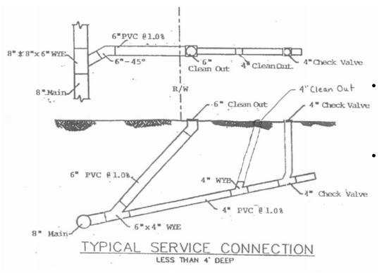
6" Cleanout = box REQUIRED! Boxes are optional on 4" cleanout & check valve.
