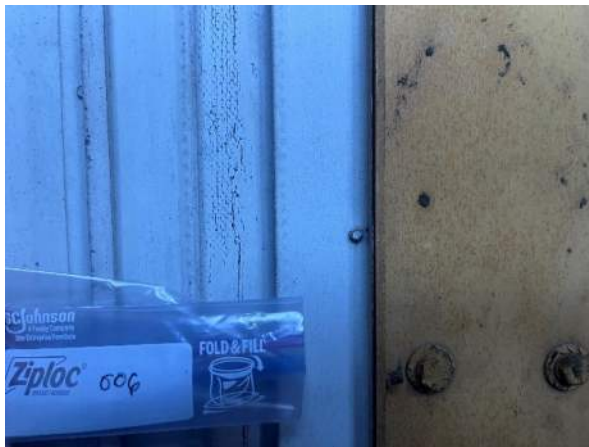
Samples # 006 / 007 Black Vibration Dampener Site/Office Building, 1 st Floor @ Generator No asbestos detected
