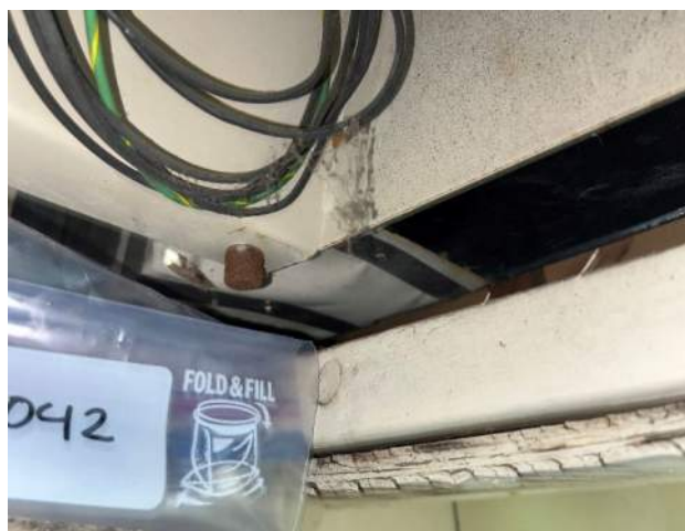
Samples 042 / 043 White Vibration Dampener Site/Office Building, 2 nd Floor Lab No asbestos detected
