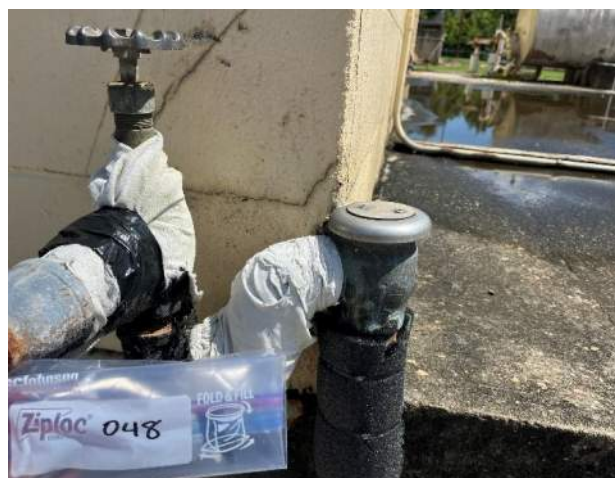
Samples 048 / 049 Black Foam w/ White Fabric Wrap Site/Office Building, Exterior No asbestos detected
