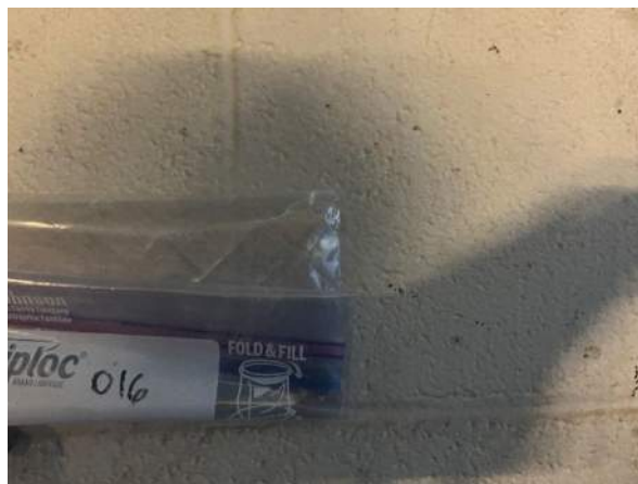
Samples 016 / 017 / 018 CMU & Paint Texture Site/Office Building, 1 st Floor No asbestos detected
