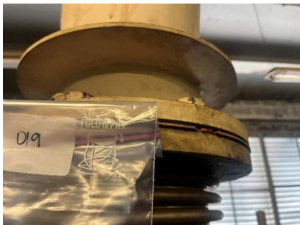
Samples 019 / 020 Orange Rubber Gasket Site/Office Building, 1 st Floor @ Blower 2 No asbestos detected
