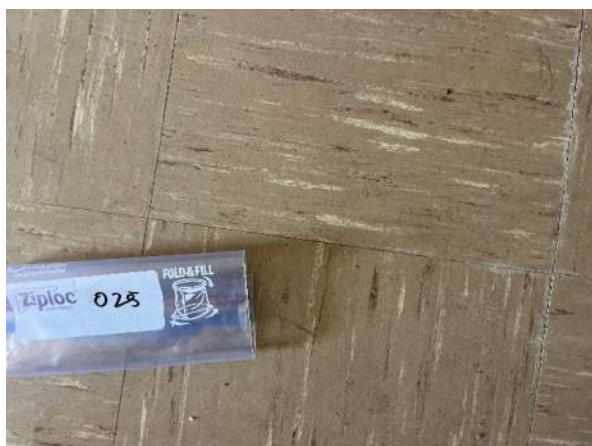
Samples 025 / 026 12" x 12" Floor Tile (tan w/ brown stripes) & Mastic Site/Office Building, 2 nd Floor Lab < 1% Chrysotile (floor tile) No asbestos detected (mastic)
