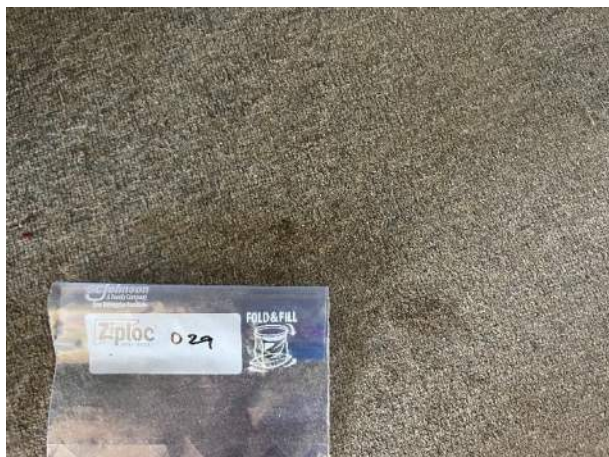
Samples 029 / 030 Carpet & Mastic Site/Office Building, 2 nd Floor No asbestos detected
